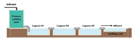
Figure 1. Schematic of the three lagoons treatment system
